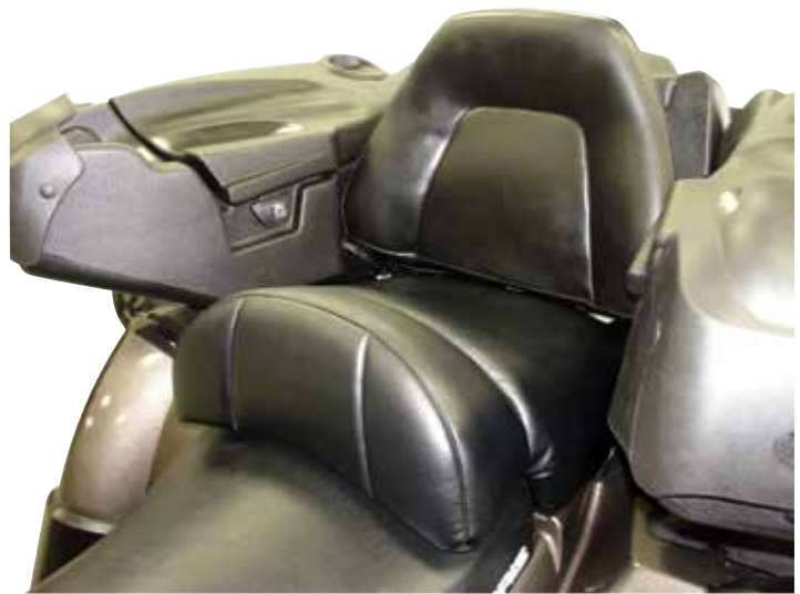
After installing the Quadrax Comfort seat adapter
