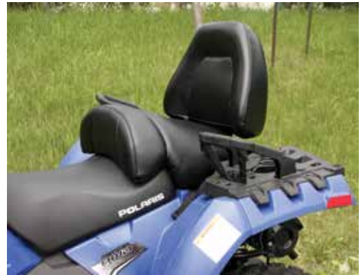
After installing the Quadrax Comfort seat adapter
